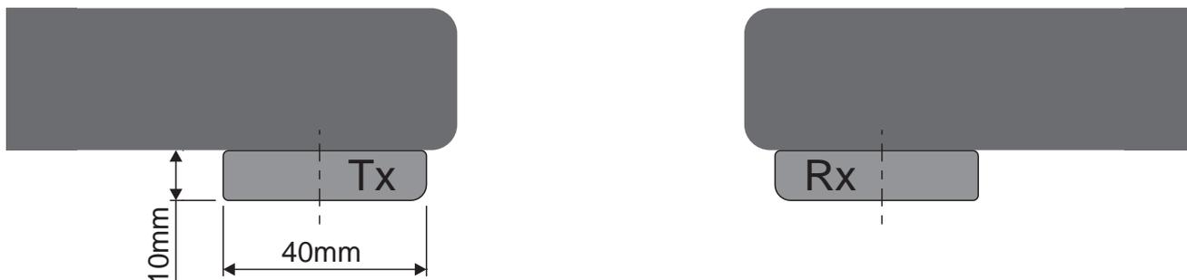
Install the Tx and Rx edges onto the doors using 5 screws to each unit.
