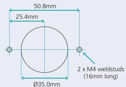
Pushbuttons with Compact 2 Micro switch body can be supplied loose or incorporated into stations. These have a vertical pitch of 50mm and a horizontal pitch of 60mm, which means the switch body can be rotated 90 degrees.
