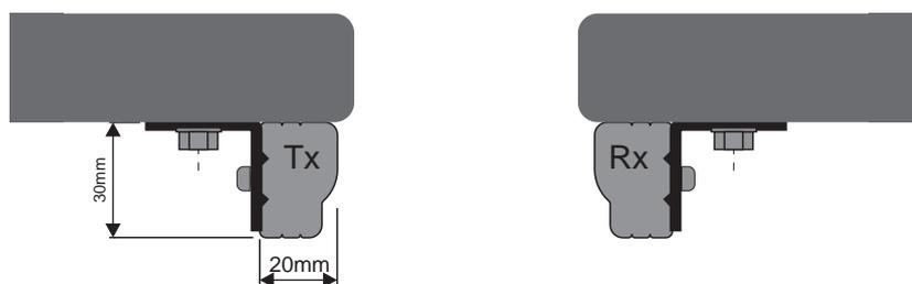
Install the Tx and Rx edges onto the doors using the mounting brackets using 5 on each edge spaced at regular intervals or as convenient if existing hole positions exist. The brackets slide into the channel from the top. Slide in all 5 before beginning to position, secure and tighten fixings
