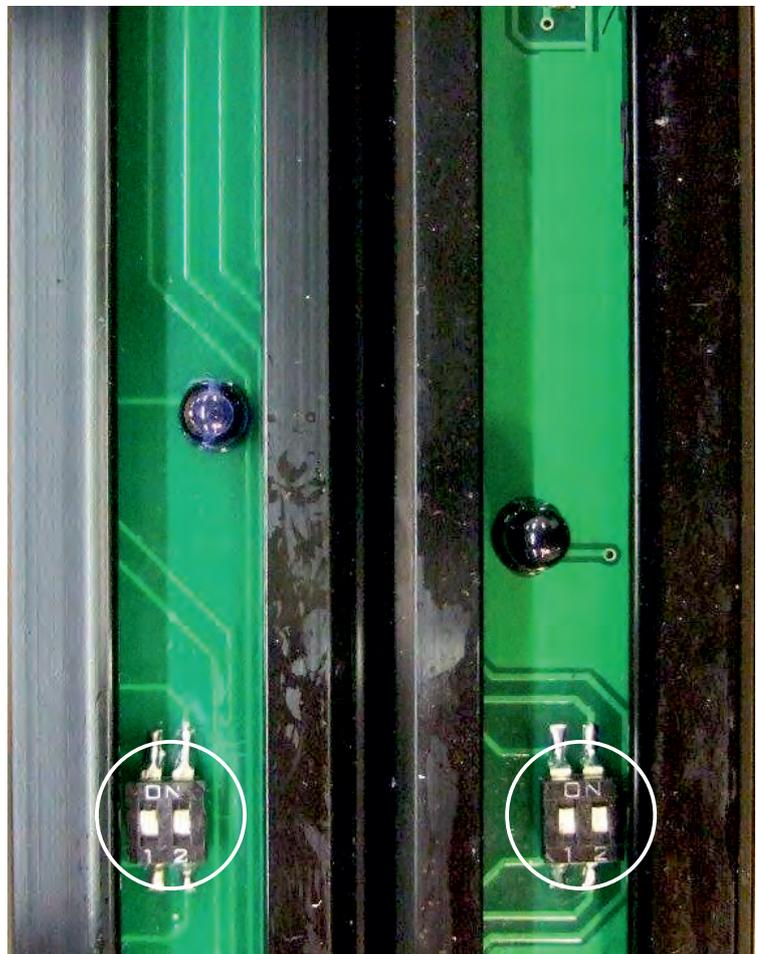
Both Rx and Tx have SILL light master controls. Switch 1 controls SILL lights. Each can be turned on or off as required. The default delivery settings have both set to the on positions (Switch 2 has no function)
